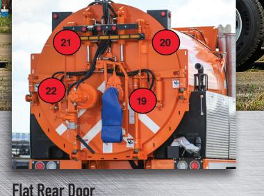
Flat-style rear door features a 6 in. Knife Valve, Arrow Stick Lighting, and Pump Off.
